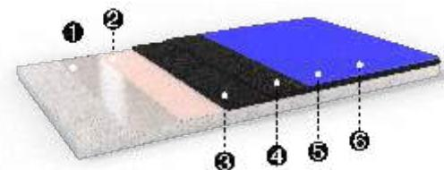
**5. ELASTOTURF 851 - Acrylic, elastic, slip-resistant, coating for sports flooring systems.**
