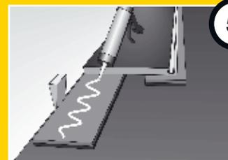
**5** In the first row, at the wall put support element under the sports parquet and glue the sports parquet on its surface with 3D 1-component poly-vinyl-acetate glue.
