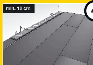
**4** The width of last row should be more or equal 10cm. If so, cut the width of the first row to be installed. If the distance between the wall (minus dilatation gap) and the last row is between 10-19cm, in this case place support element in the aperture and glue the parquet cut on the surface of support element with 1-component poly-vinyl-acetate glue.
