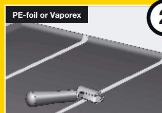
**2** If the moisture content of the sub-floor is higher than 1,8CM% but less than 5CM%, always use Grabo Vaporex damp-proof underlay floor. If the moisture content is less than 1,8CM% you can put PE-foil under the sports parquet.
