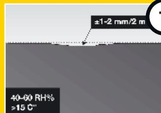
**1** Relative humidity between 40 and 60% and temperature minimum 15C° must be ensured during laying and use. The sub-floor flatness tolerance should be max. 2 mm/meter.
