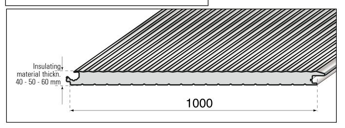
Alutech is the system with high density polyurethane foam insulated sandwich panels, designed for covering and cladding the perimeter walls of houses and industrial constructions. Alutech Wand is designed to make walls with the external surfaces shaped to fit longitudinally and fitted with concealed fixing mechanisms.
